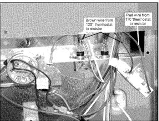
**15.** Connect the #5 (318052586 - Brown) wire to the remaining terminal of the 120° thermostat. Connect the other end to the "NO" terminal of the new switch
